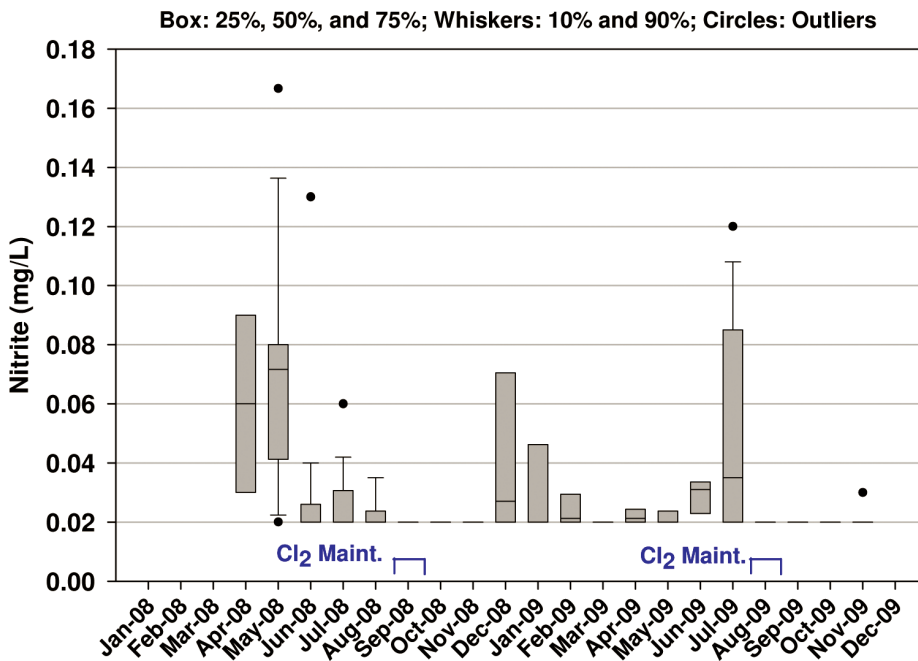
Figure 5: Utility Distribution Network Routine Site Monthly Average Nitrite (2008–2009)
